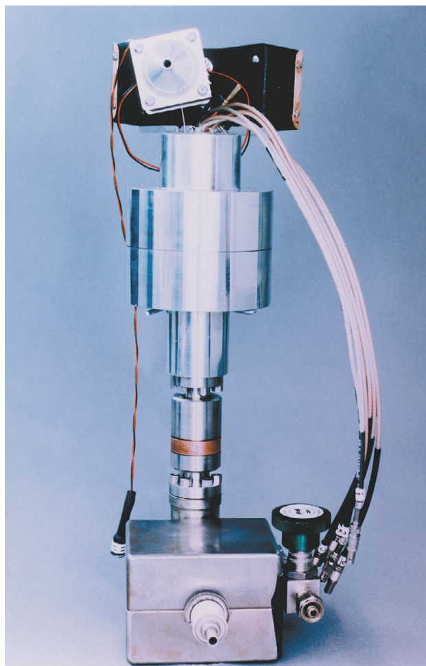
Figure 1. This view of the miniature mass spectrometer outside its suitcase shows the small magnet in the middle of the cylinder.
