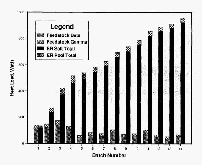
Fig. 1. Batchwise Heat Contents in the Feedstock and Cumulative Heat Load to the Electrorefiner
