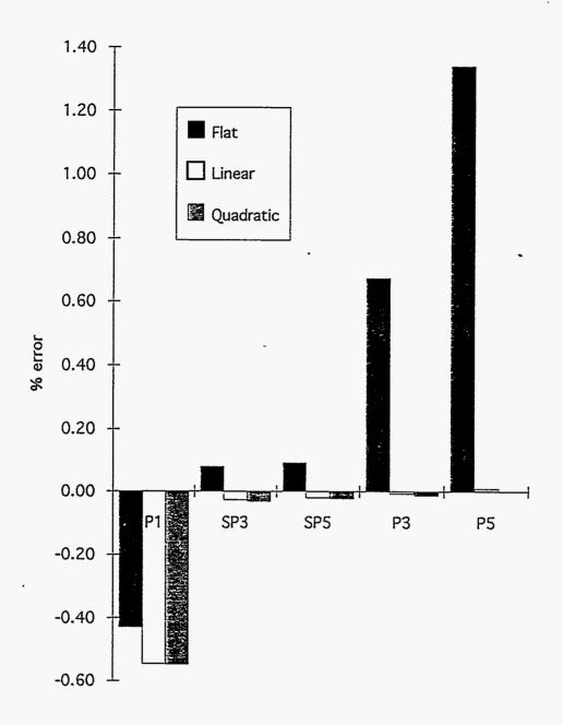
Figure 1. Eigenvalue Errors for the "Rods In" Takada Benchmark II (reference k = 0.95954)
