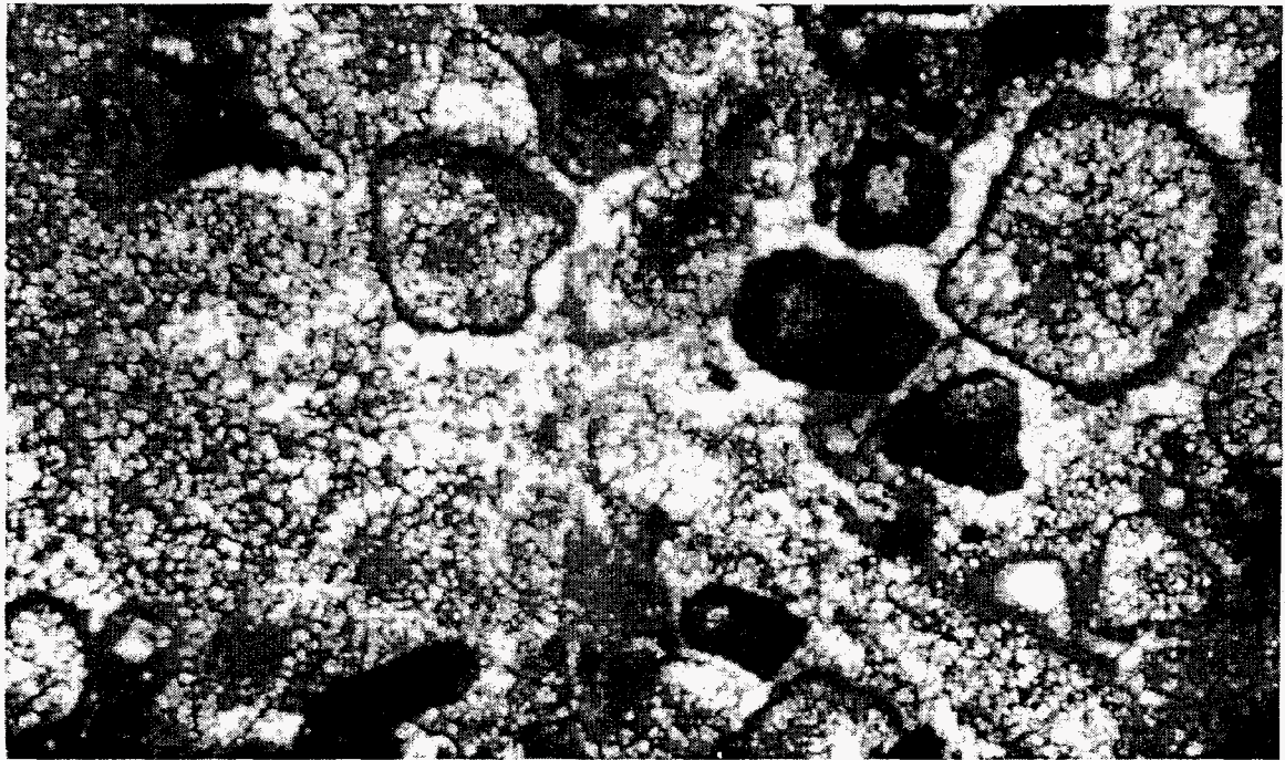
Figure 5. Photomicrograph of agglomerate in the loopseal area of a circulating fluidized bed combustor. Notice that the area between the particles has been filled with calcium sulfate. See text for discussion. (Field of view across the bottom of the photo is 0.7 mm).
