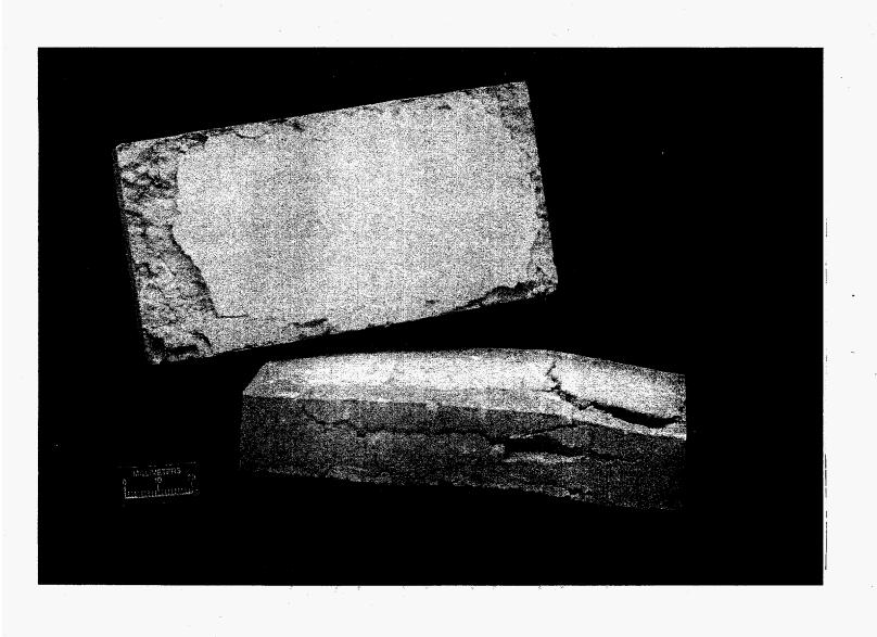
Fig. 5. Brick waste forms produced by the TIDE process.
