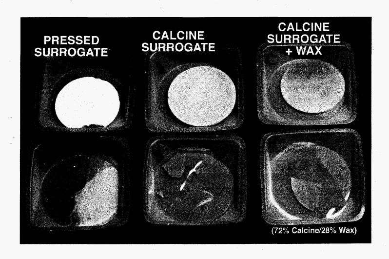
Fig. 4. Surrogate waste [pressed at 4500 lb/in.² (psi)]. Top row: pressed waste form; bottom row: fragments of pressed waste form placed in water.
