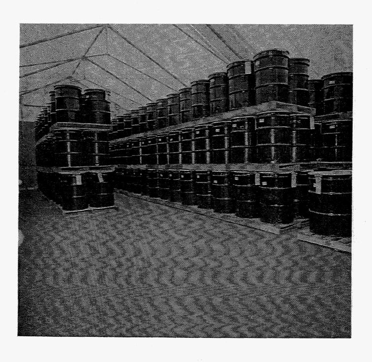
Fig. 2. Typical storage array for as-generated raw sludge.
