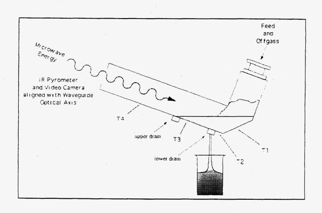
Fig. 8. Continuous-feed microwave melting apparatus (courtesy of T. L. White).
