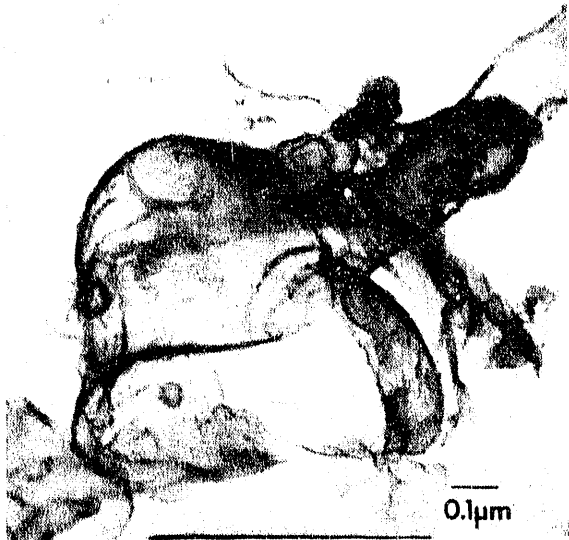
Fig. 25. Ribbon-Like Clay Colloids from IV9165-A-91. The contrast is due to parts of the colloid being at the Bragg reflection position.
