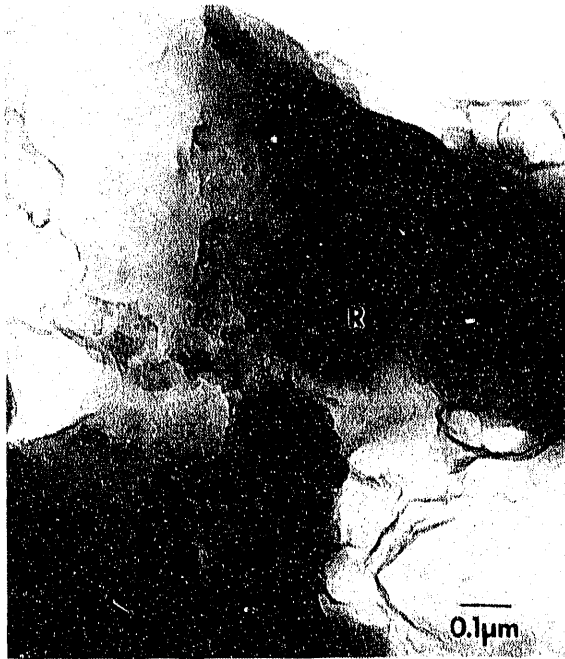
Fig. 28. Brightfield Micrograph of a Particle of Rutile Attached to a Clay Colloid from Sample DP3
