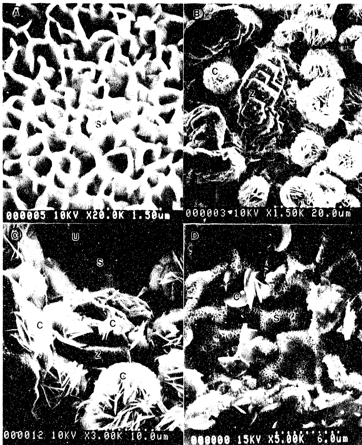
Fig. 32. SEM Micrographs from the Bright Part of the IVE202U-14-1-2 Sample Surface. Letters marked on the micrographs represent: S--smectite; Z--zeolite; C--calcium silicate; C*--calcium silicate with aluminum; and U--uranium silicate.
