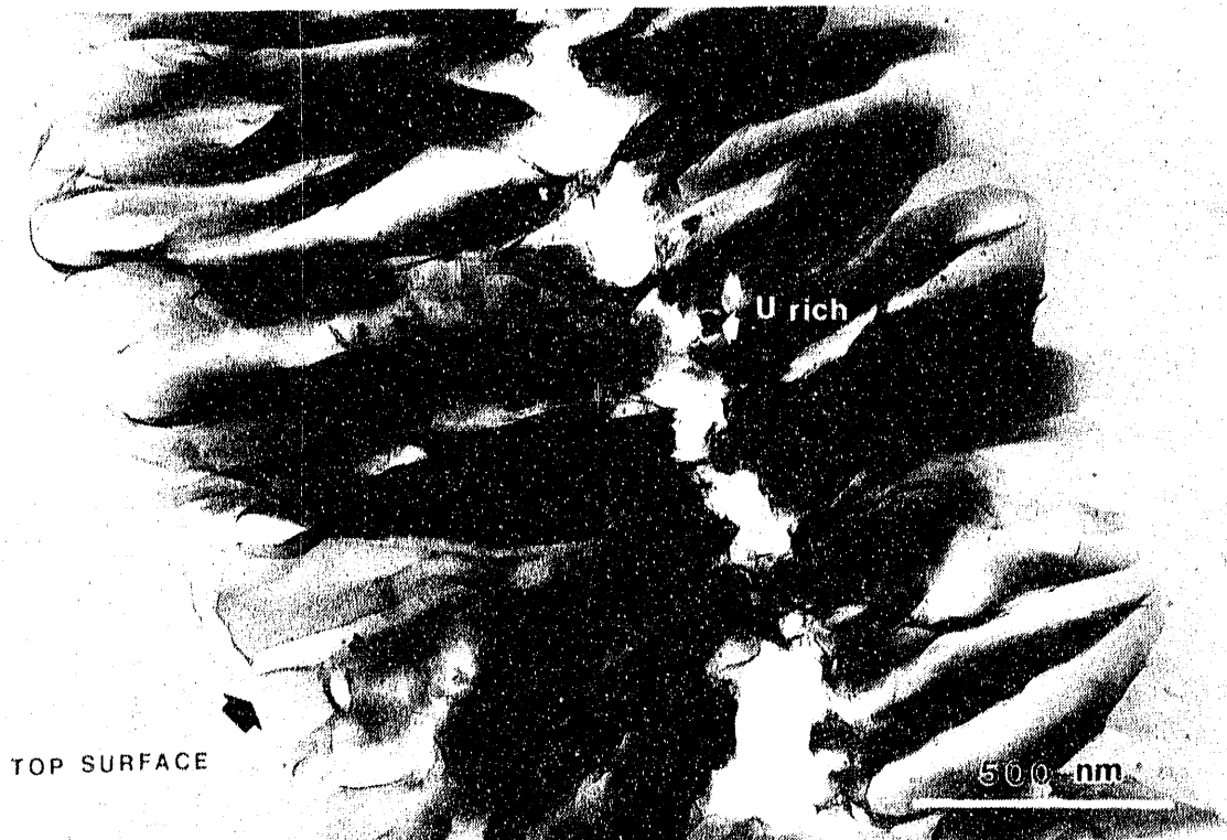
Fig. 45. TEM Micrograph of the Alteration Layer on the Surface of B-82 Sample. Note: There are two layers of smectite; small uranium-rich particles are observed at the layer interface.
