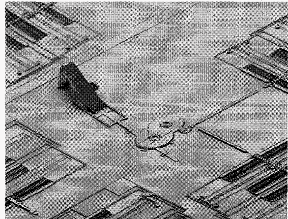
Figure 4. Polysilicon mirror driven out of plane using a microengine, microtransmission and rack and pinion assembly.
