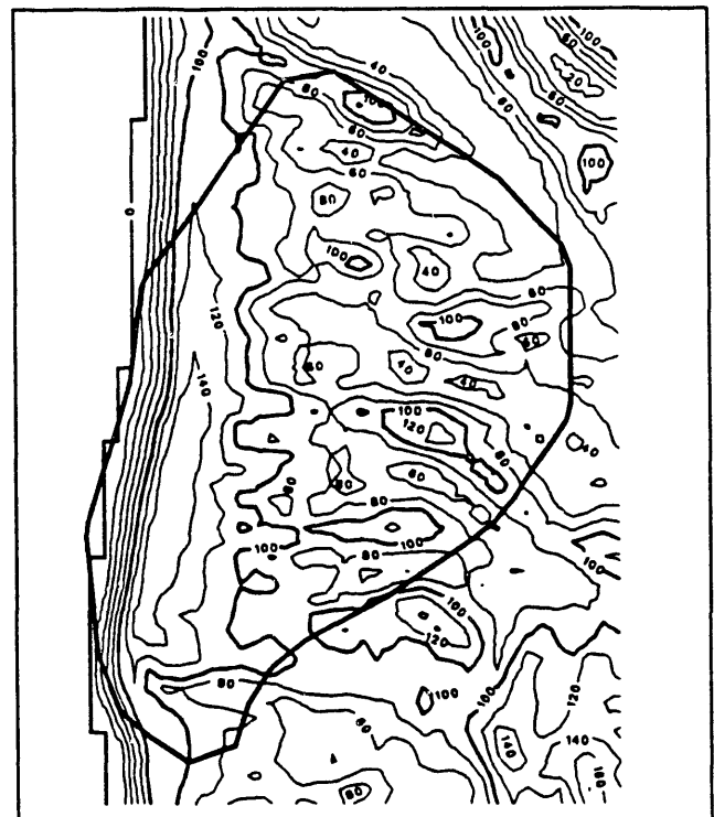
FIGURE 5. Example of Contour Map Showing the Thickness of Tiva Canyon Welded (TCw) Unit and the Repository Boundary
