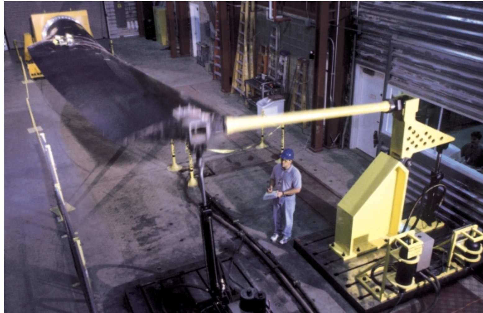
A National Wind Technology Center test engineer observes a fatigue test of a Zond Z-48 blade under two-axis loading to simulate thrust and torque. Blade tests conducted on the Zond Z-750 kW Series will lead to wind turbine type certification.
