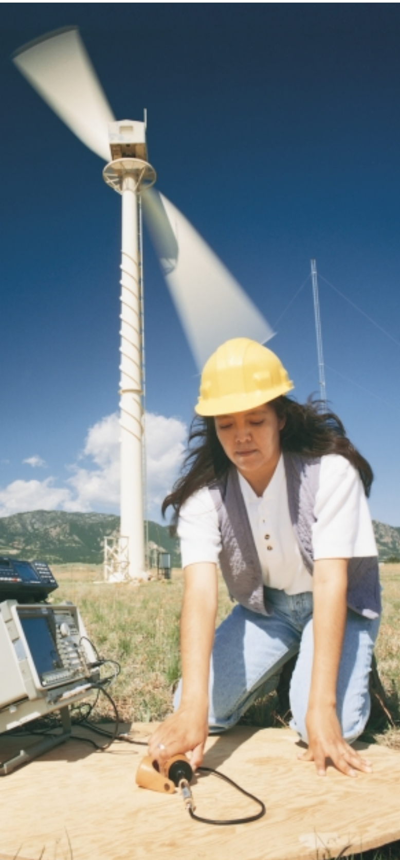
Acoustic noise measurements are not required for type certification but many local authorities require them. The National Renewable Energy Laboratory received accreditation in 1998 to perform acoustics tests on turbines.
