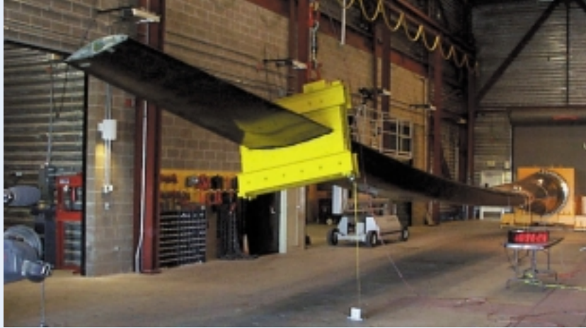
The Zond turbine blade under test at the National Wind Technology Center.
