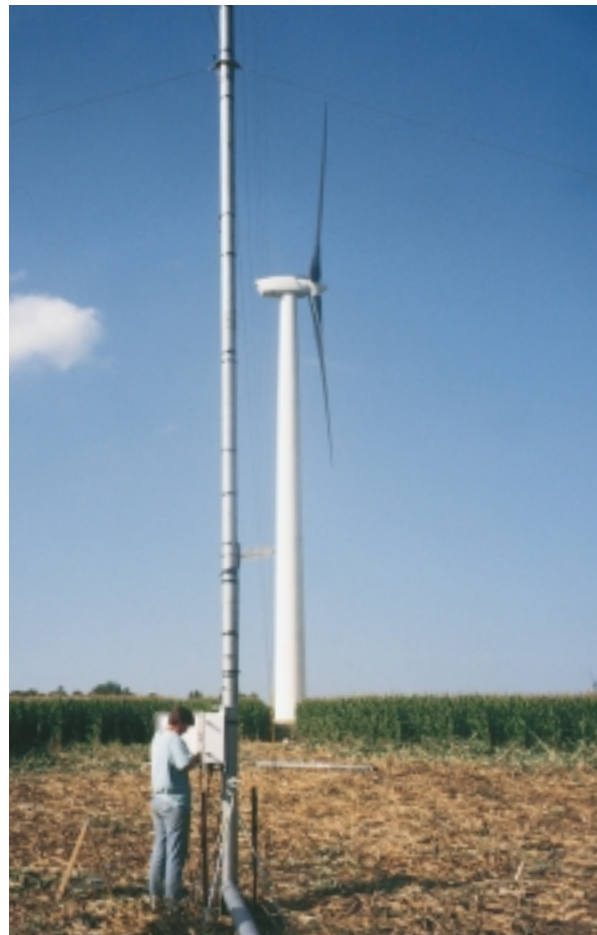
A National Renewable Energy Laboratory engineer installs an anemometer near a Zond Z-48 turbine at the Lake Benton I Project in Minnesota. The anemometer was installed as part of power performance testing of the Z-48 turbine, which will lead to type certification of the Z-750 kW Series.
