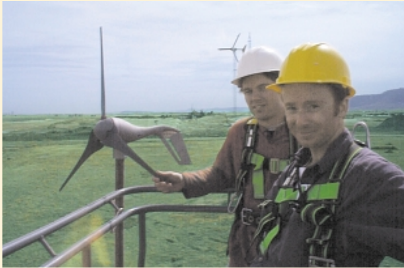
Southwest Windpower employees Rusty Knowler, mechanical engineer (left), and Tim Sasseen, director of research and development, with the Southwest Windpower Air 403 battery-charging wind turbine at the National Wind Technology Center. The turbine will operate under test for 2500 hours as part of wind turbine type certification.
