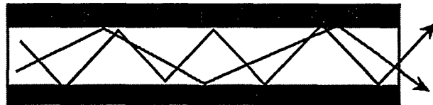
Figure 3-2. Optical fiber guides light
