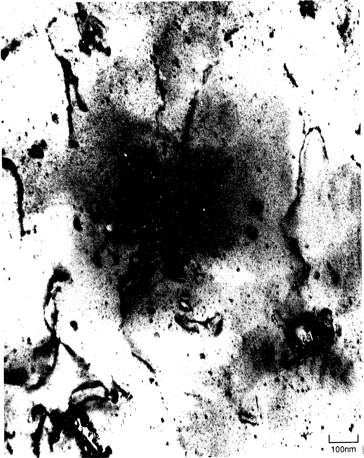
FIGURE 8.25. Microstructure of Grain Interior Near the Mid-Radius of Section 104-MKP109-S. ( Particle (A) surrounded by dislocation tangles.) (Neg. LT 1157)
