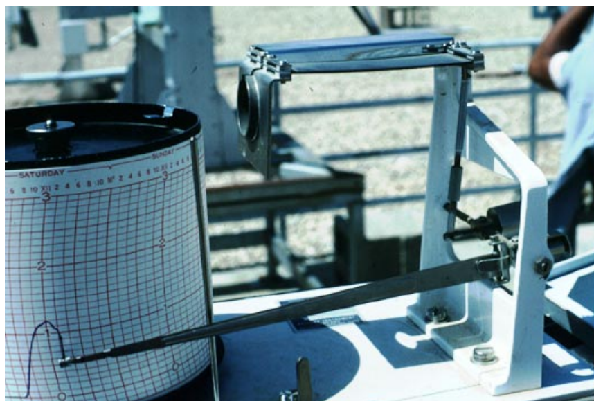
Figure 7-2. Belfort actinograph with cover removed showing pen linkage to bimetallic strips at top
