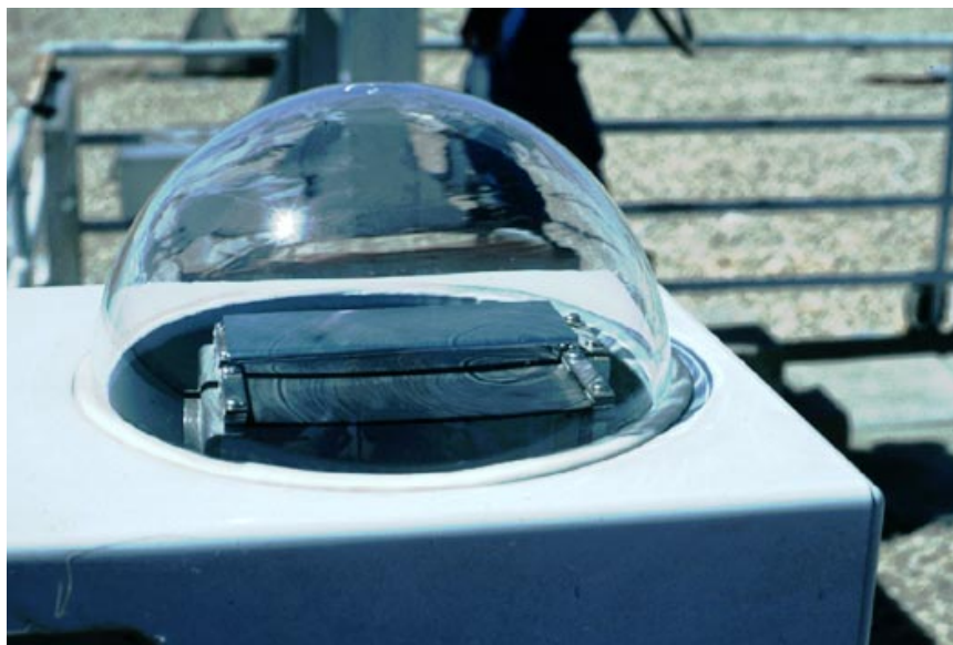
Figure 7-1. Bimetallic strips under dome of a Belfort actinograph (shaded strip toward the back)
