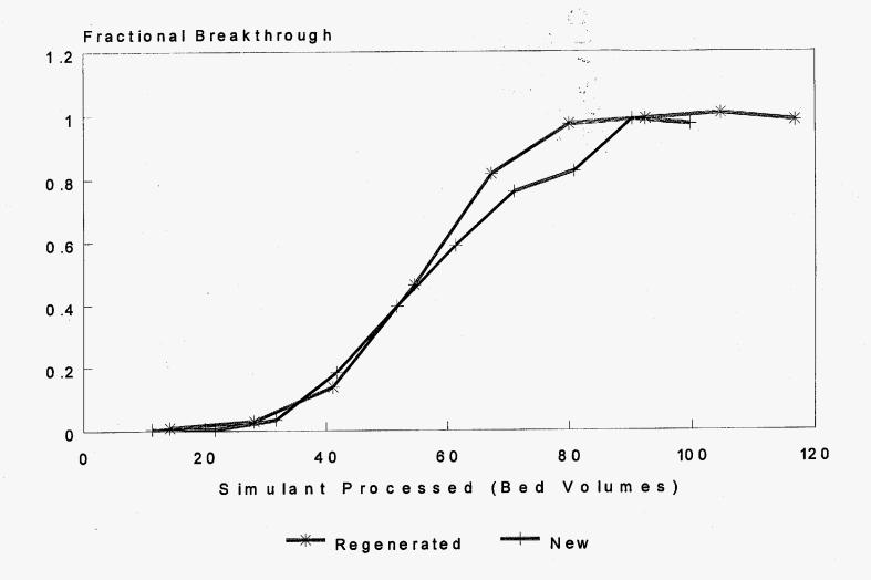
Fig. 7. Treatment of INEL simulant. New vs. regenerated SuperLig 618.
