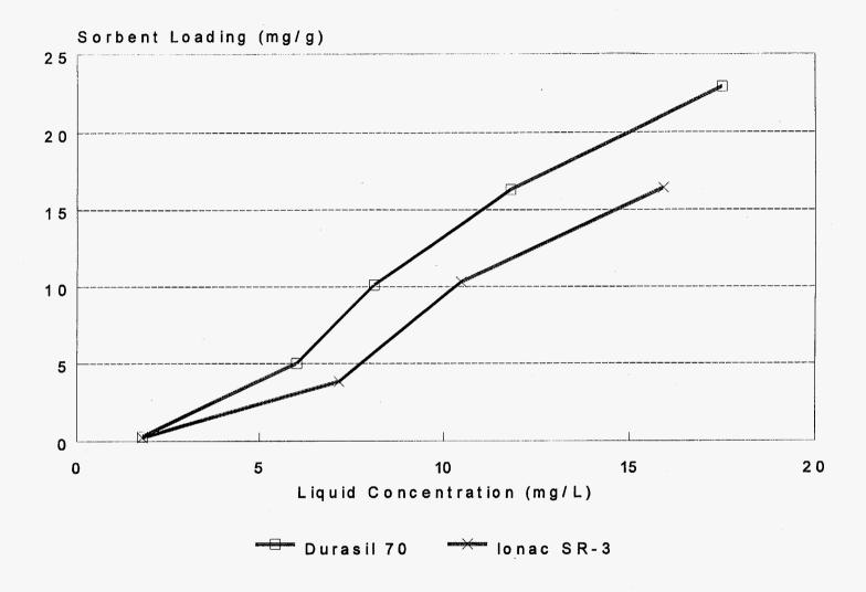
Fig. 3. Batch isotherm results in Y-12 lithium hydroxide solution. 24-h batch tests, 28 mg/L Hg initially.
