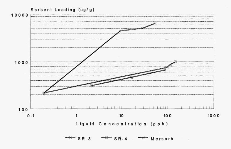
Fig. 2. Batch isotherm results in Y-12 sump water. 24-hr batch tests, 220 ppb Hg initially.
