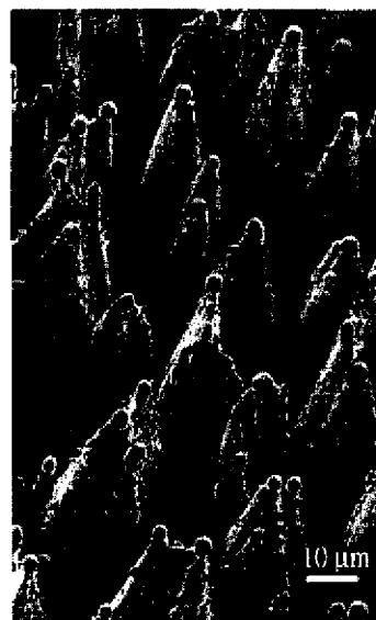
Figure 6. Silicon microcones joined by walls, produced by 2040 laser pulses at 1.5\text{ J/cm}^2 in SF 6 . (Ref. 35)
