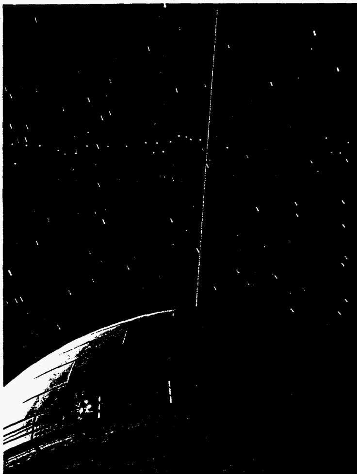
Figure 1. Propagation of the sodium guide star laser from the 3 m Shane dome at the Lick Observatory.
