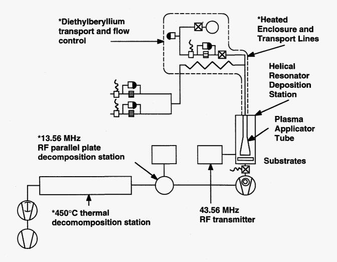
Figure 1. Schematic component diagram of the organoberyllium plasma polymerization system. Sections labeled with a "\*" are new or modified from the standard plasma polymerization configuration.
