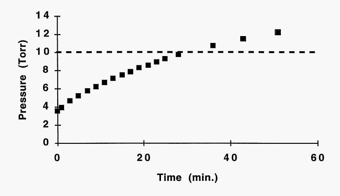
Figure 3. Plot of the diethylberyllium bubbler pressure as a function of time after reaching a steady state oven temperature of 62°C and freshly evacuating the head space.
