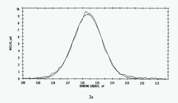
Figure 2. XPS spectra for (a) beryllium, (b) carbon, (c) oxygen and (d) silicon in beryllium doped plasma polymer.
