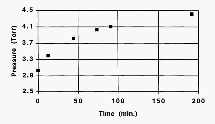
Figure 5. Plot of the diethylberyllium vapor pressure versus time at 42°C. The container was evacuated and the pressure allowed to come to equilibrium again.
