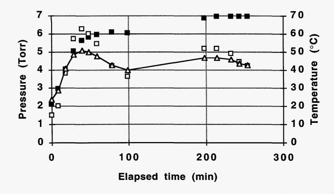
Figure 4. Plot of the diethylberyllium vapor pressure (experimental and calculated) and source oven temperature as a function of time.
