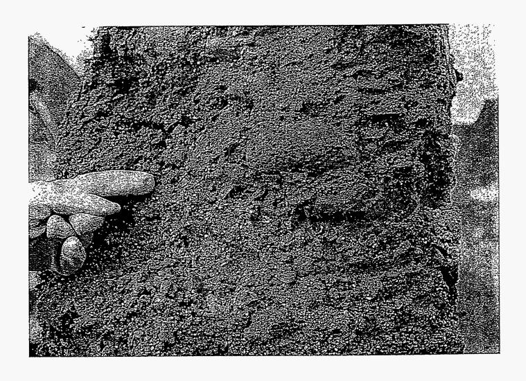
Figure 2. Excavated portion of the CS grouted soil. Note the extreme heterogeneity of the soil, indicated by the particle size and the appearance of the granular material.
