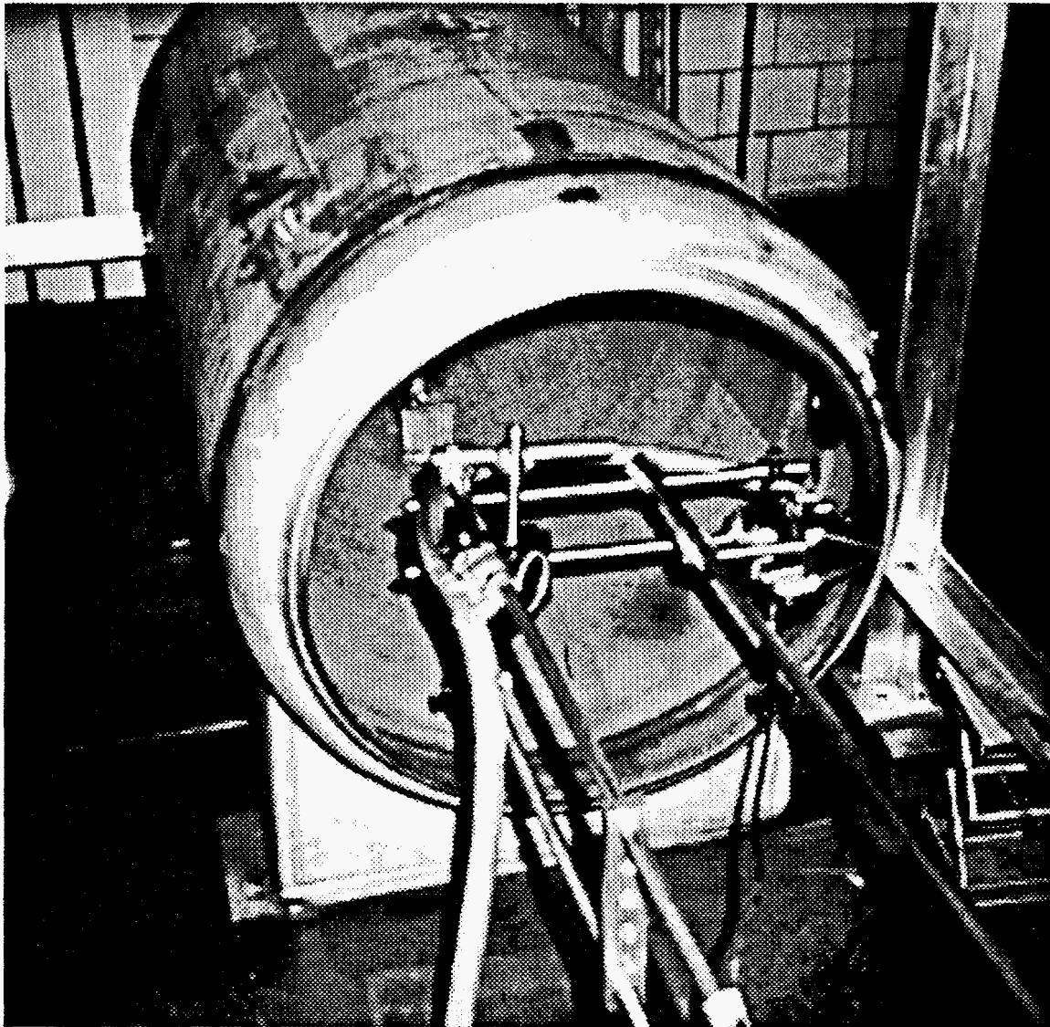
Figure 7. Optics and cleaning cell deployed for interior cell wall cleaning.
