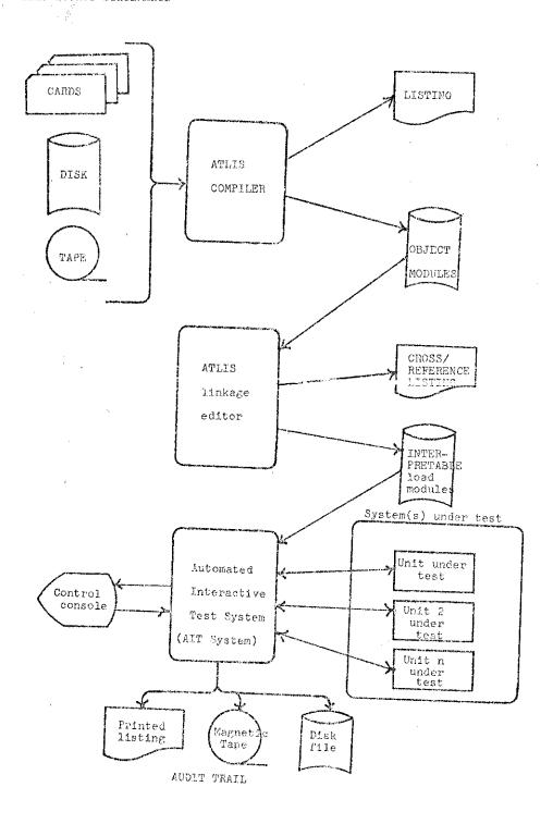
Fig. 1--An overview of the automated interactive test system.
