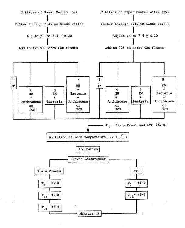
Fig. 5--Experimental protocol for analyzing anthracene or pentachlorophenol (PCP) in the experimental water with addition of glucose.
