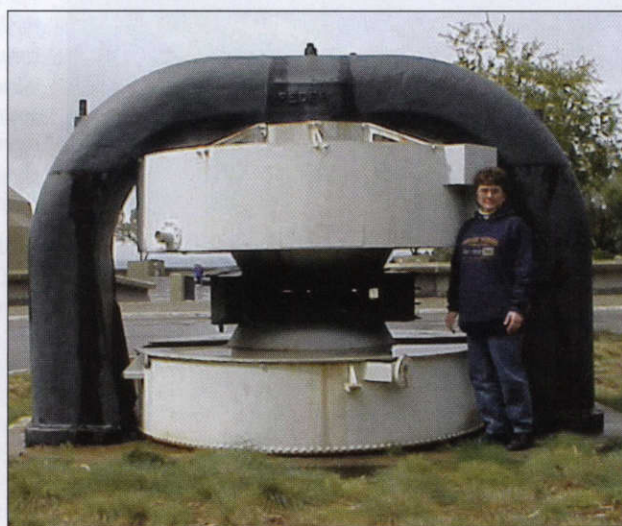
ABOVE: Figure 10. The magnet used for the 27-inch cyclotron (operational 1932), then modified to the 37-inch cyclotron (operational five years later), is now standing outside the Lawrence Hall of Science. The magnet, originally built for power communication between the U.S. and Europe in World War I, was acquired by Lawrence as war surplus.
