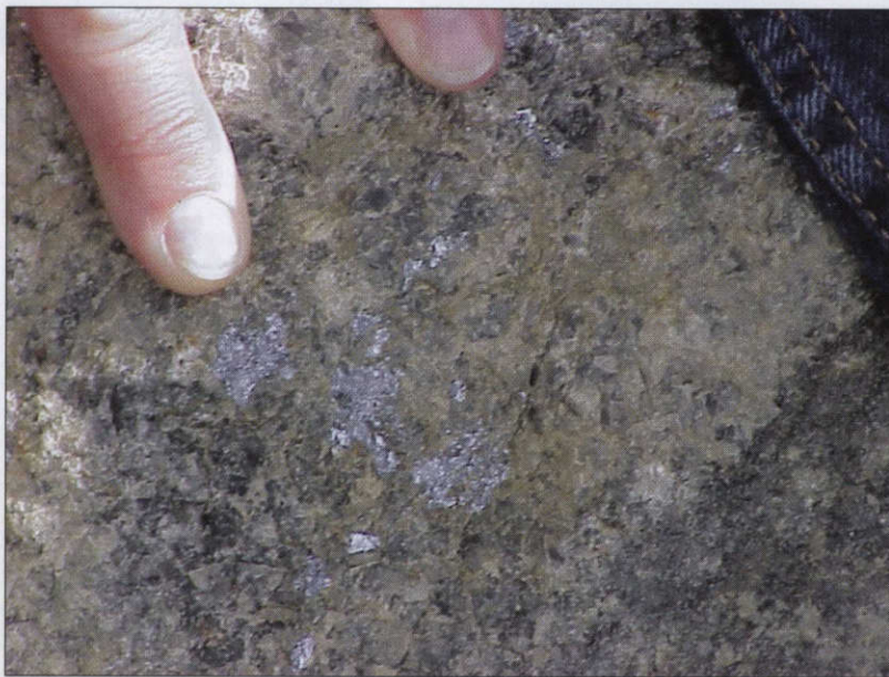
RIGHT: Figure 5. The talus scattered about at Knaben, Norway—900-million-year-old Precambrian granitic gneiss—is profuse with molybdenite that looks like splashes of solder. The molybdenite is rich in rhenium, with concentrations as high as 7.5 ppm. 7
