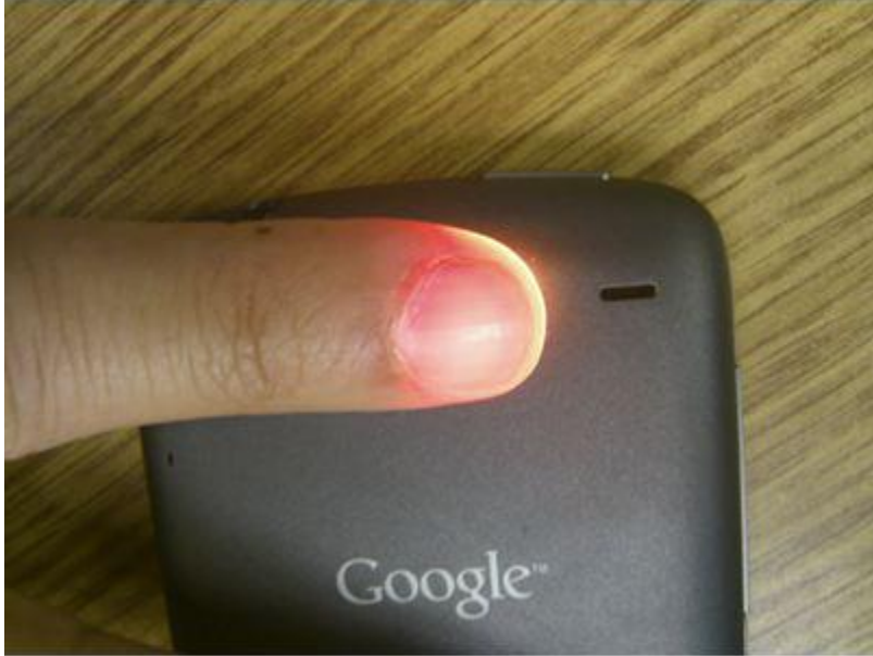
FIGURE 8.4. Using smartphone for Taking Reading for Heart Rate. The finger is placed on the mobile camera lens.
