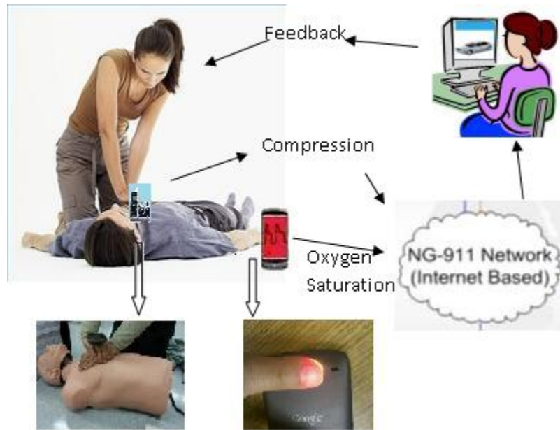
FIGURE 3.2. CPR and Its Evaluation. The compression frequency, depth and the oxygen saturation levels are reported to the 9-1-1 operator. The person giving CPR has a phone tied to the hands, as shown in the picture below the arrow. A smartphone is also placed near the hand of the person receiving the CPR with finger on the camera lens as shown in the second picture below the arrow.
