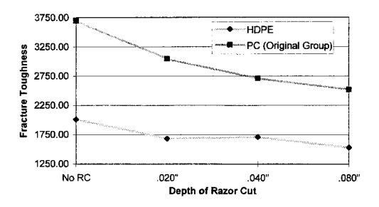
Figure 4.1 Fracture toughness versus depth of razor notch.
