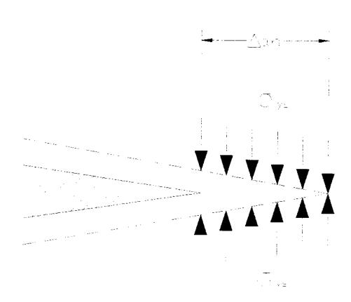
Fig. 2.2 Plastic zone according to Dugdale's model.
