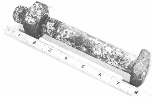
Fig. 24 Photograph of broken bolt on stabilizing band.
