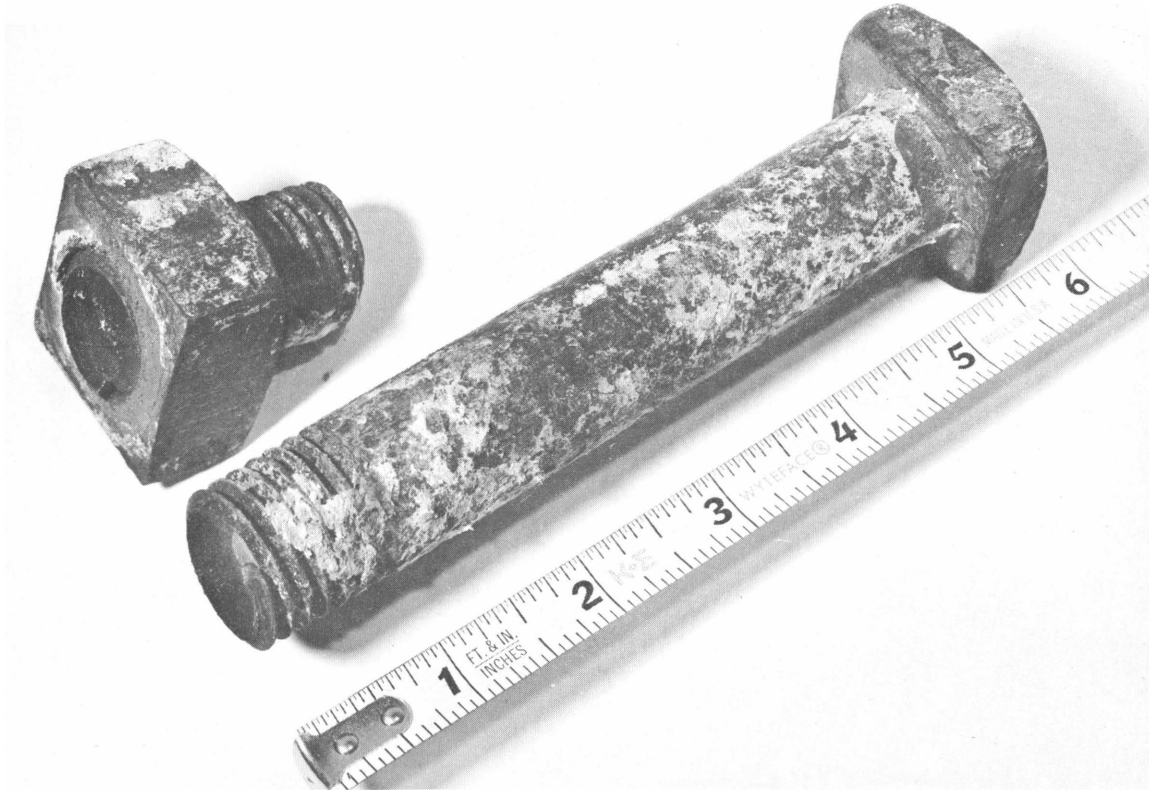
Fig. 22 Photograph of broken stabilizing-band bolt.
