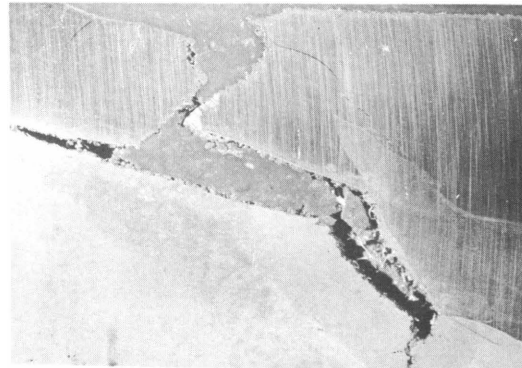
Fig. 52 304L cladding crack at the edge of the weld, 14X, electrolytic etch. The weld is the thicker material.
