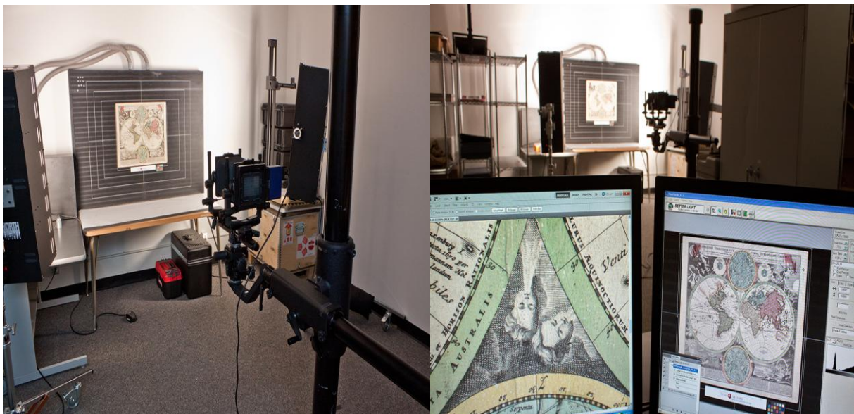
Figure-1 Capturing Digital Images of the Maps with the Better Light Scan Back System
