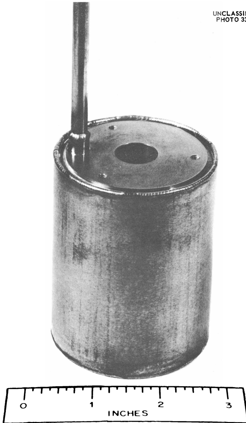
Fig. 75. High-Temperature Radiation-Resistant Differential Transformer.
