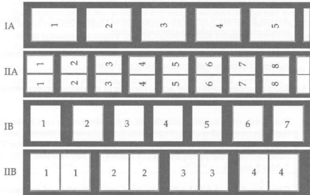
Figure 1.2: Microfilm page position codes. (RLG Guidelines, 2003)
