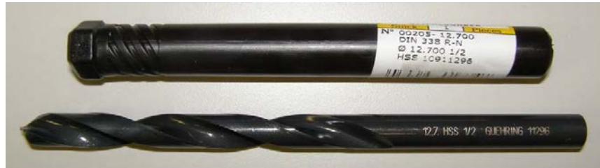
Figure 1: High Speed Steel Drill Bit (Source: University of North Texas, Manufacturing Engineering Laboratory)
