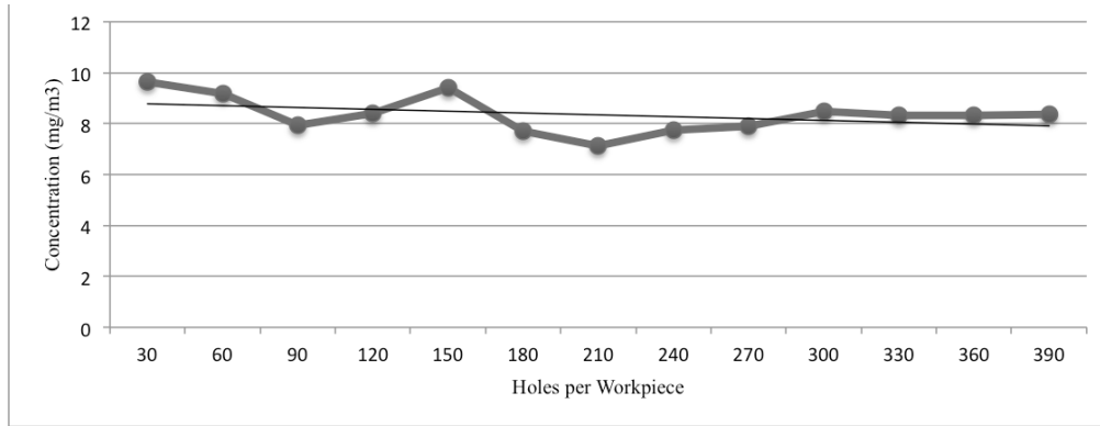
Figure 15 (a): Concentration Levels at 100 SFM and Feed of 0.004 IPR
