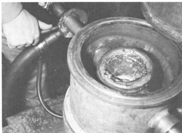
Figure 147. —Furnace interior showing skull in position.
