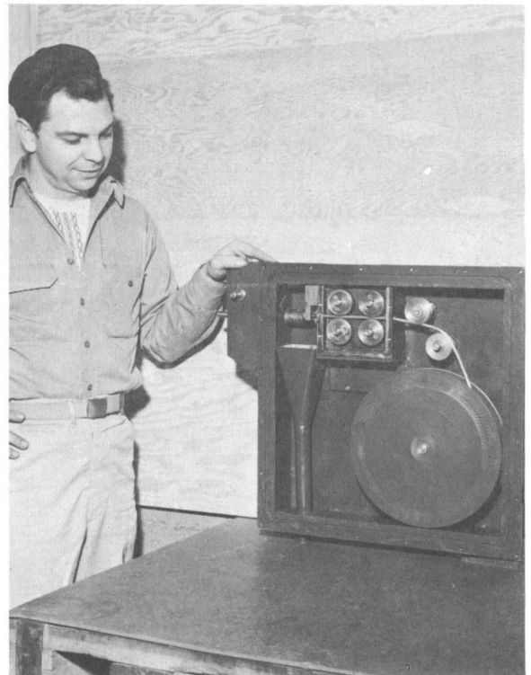
Figure 4.—Automatic tin-chopper mechanism.
