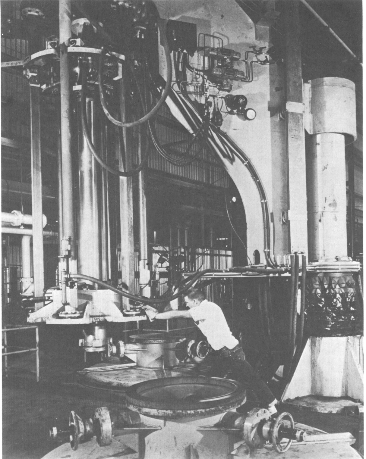
Figure 15.—An example of an electrode-drive assembly—Titanium Metals Corp. of America.
