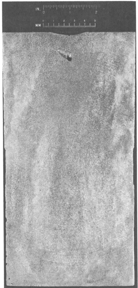
Figure 20.—Longitudinal ingot section.
