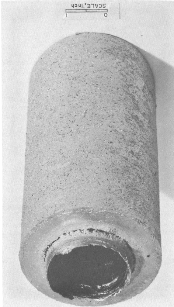
Figure 167.—A typical horizontal-axis casting, as removed from the mold.
