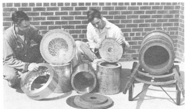
Figure 99.—Typical centrifugal castings of titanium produced in mold on right.
