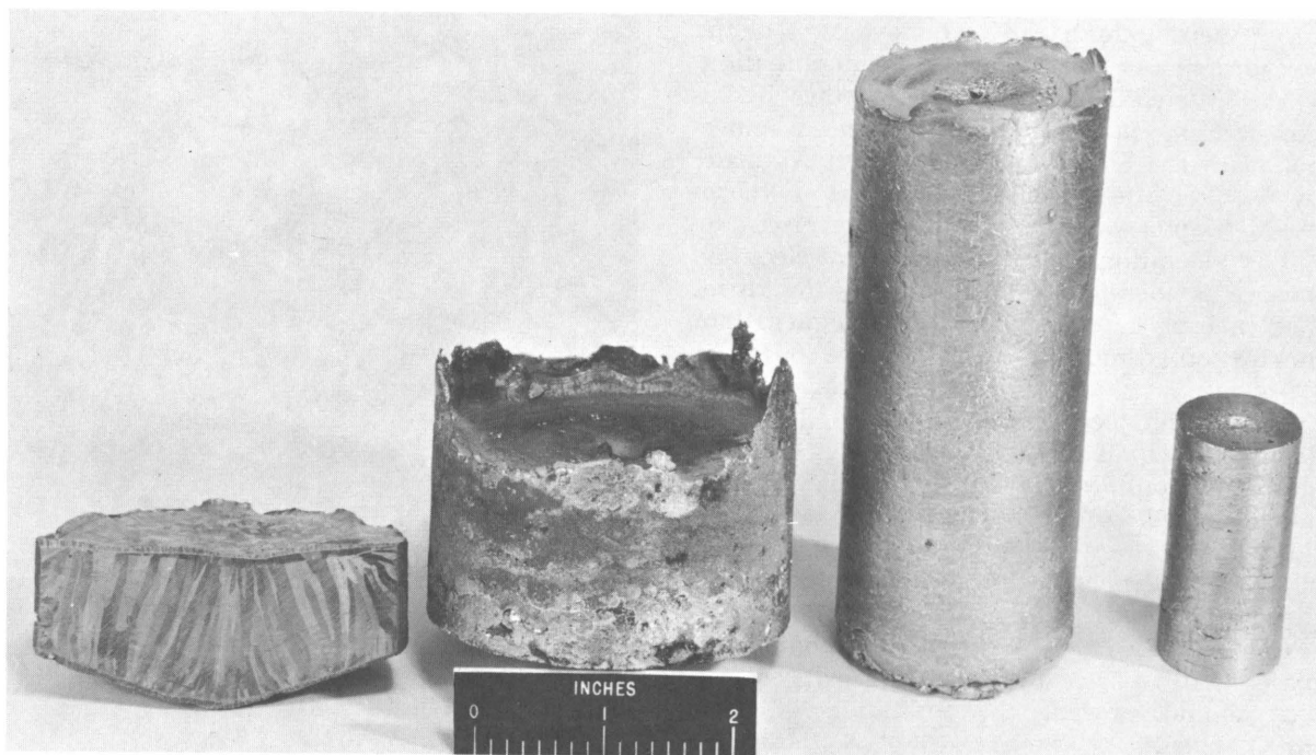
Figure 18.—Typical as-cast chromium ingots.
