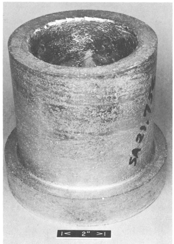
Figure 23.—Electron-beam furnace component of cast copper.
