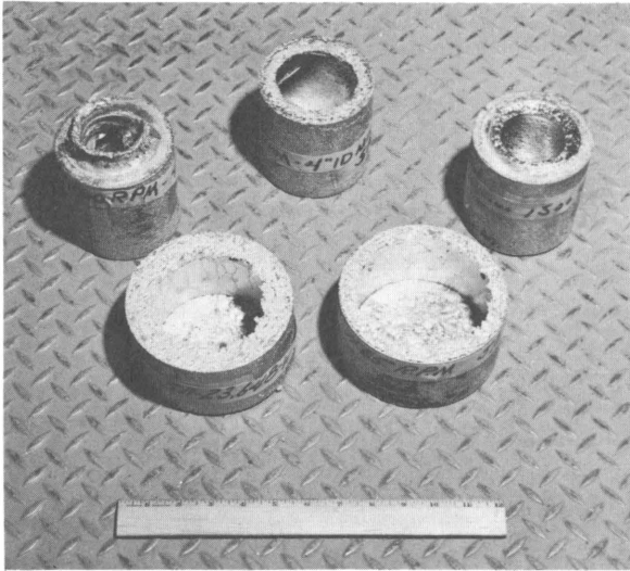
Figure 165.—Group of spin castings: Note the indications of hot tearing on the inner walls, bottom left.
