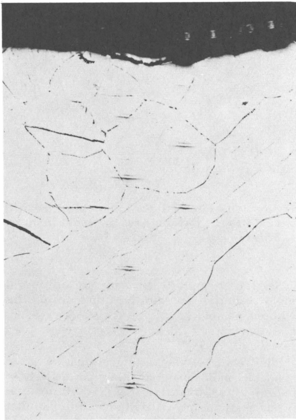
Figure 141.—Microstructure of hafnium cast in mold material BW, near cast surface (SA 21,709). Etch: 45 ml H 2 O, 45 ml HNO 3 , 10 ml HF ( \times 100 ).
