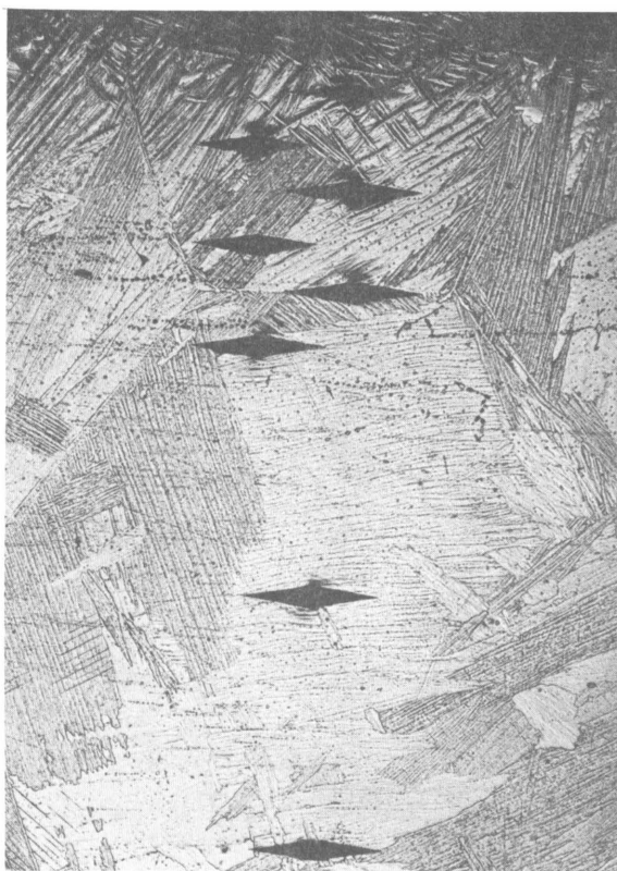
Figure 131. —Microstructure of casting SA 22,511 in area of Knoop traverse. Knoop hardness indentations made with 1 kg load. Etch: 45 H 2 O, 45 HNO 3 , 10 HF (× 50).
