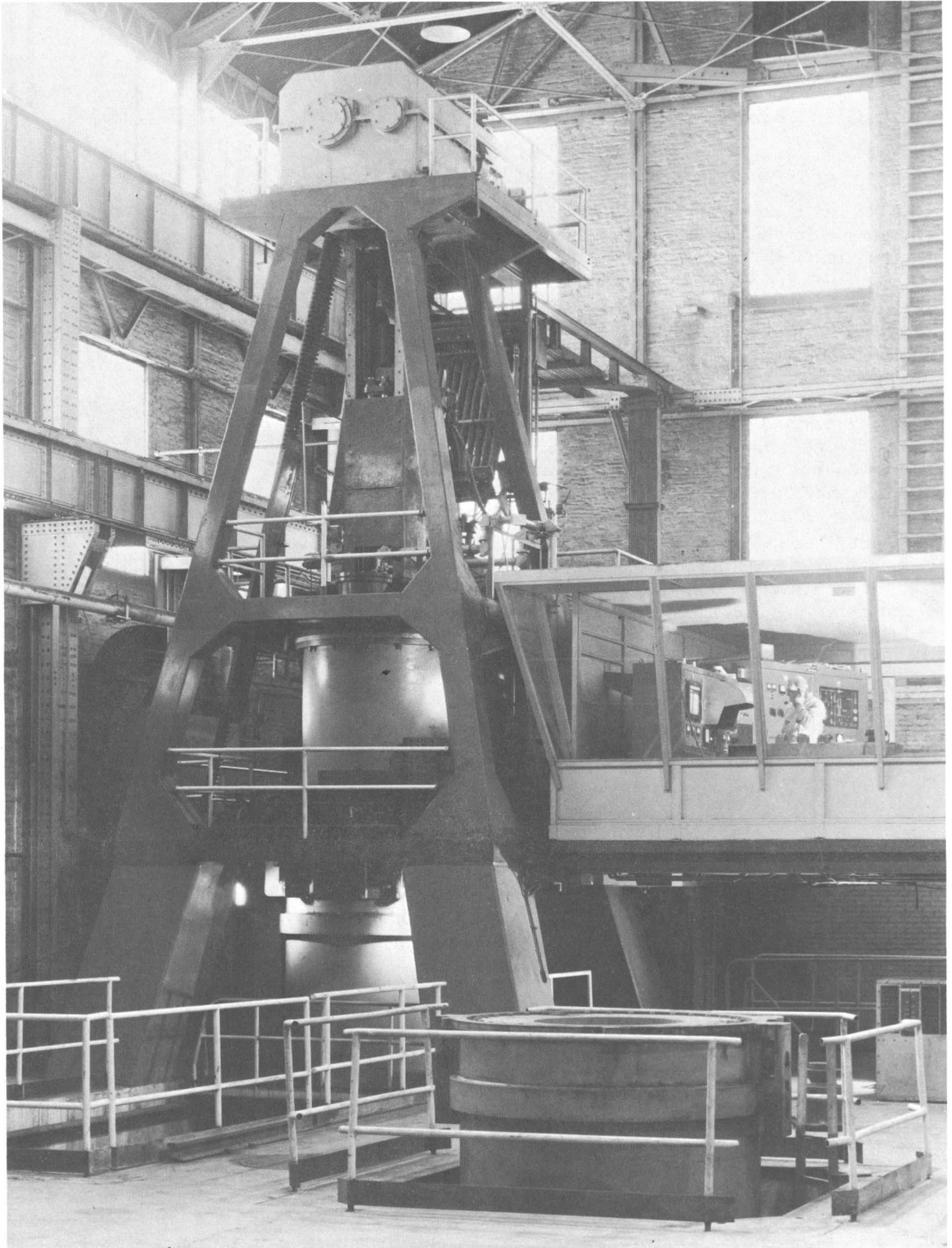
Figure 12.—The Midvale-Heppenstall furnace capable of producing 60-in-diam ingots.
