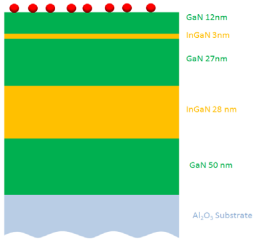
Figure 5.5.1 3 nm InGaN SQW with gallium droplets
