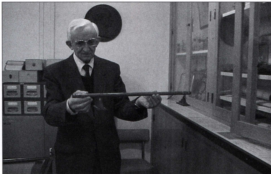
Figure 4. Le Professeur émérite Jacques Rivet holding a special metal tube constructed by Henri Moissan used to study elemental, gaseous fluorine. Capped with transparent, inert fluorite caps, the tube allowed Moissan to observe for the first time that the color of elemental fluorine is yellow.
