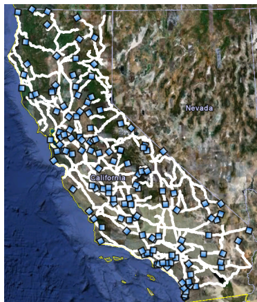
Figure 3.5. 136 simulated vehicles on the California road network for 90 minutes. Each blue square represents the vehicle destination and the white lines trace all the routes by the end of the dataset.
