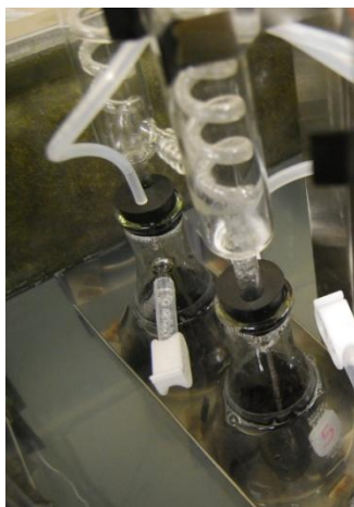
Figure 9.4 Composting bioreactor showing the inlet channel connected to a stainless steel tube.
