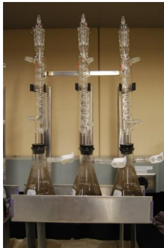
Figure 9.5 Composting bioreactor showing the air-cooled Graham condenser.
