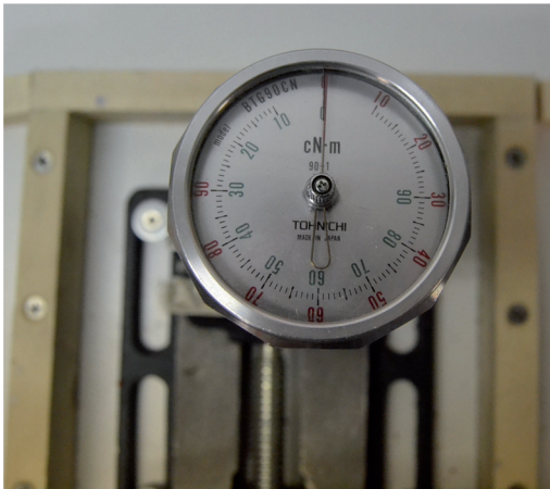
Fig. 2. Implant primary stability measured by peak insertion torque with a manual torque wrench.
