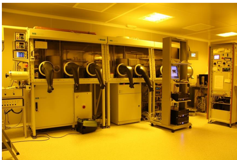
Figure 7. MBraun glove box installed inside the clean-room at the Instituto de Ciencia Molecular (ICMol) of the Universidad de Valencia where all the devices were prepared and characterized.
