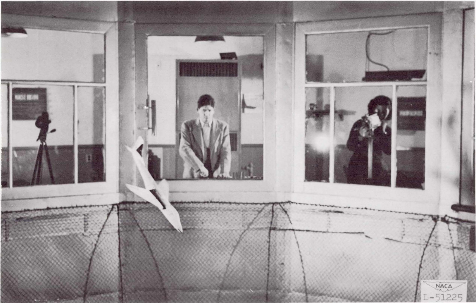
Figure 7.- Model A spinning in the Langley 20-foot free-spinning tunnel.
