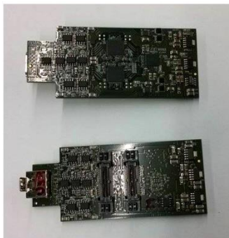
Figure 4.39: Picture of the FADC Mezzanines. Up) Top view. Down) Bottom view
