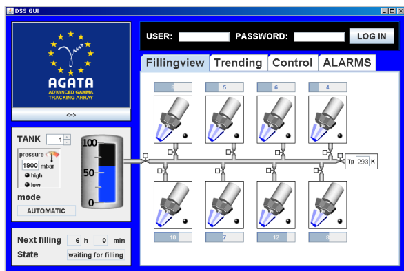
Figure 22: (Colour online) The graphical user interface of the AGATA detector-support system showing the autofill page. The autofill manages detectors in groups of 8 units. On the left hand side of the figure, the level of liquid in the main supply tank is shown as well as its internal pressure and the time remaining to the next programmed fill. On the right hand side, the colour of the detector endcap gives an indication of the detector temperature (blue for cold, orange for warming up, red for warm). Trending (real-time plot of any variable parameter), Control (parameter setting) and Alarms (alarm status) pages are also accessible from this GUI.
