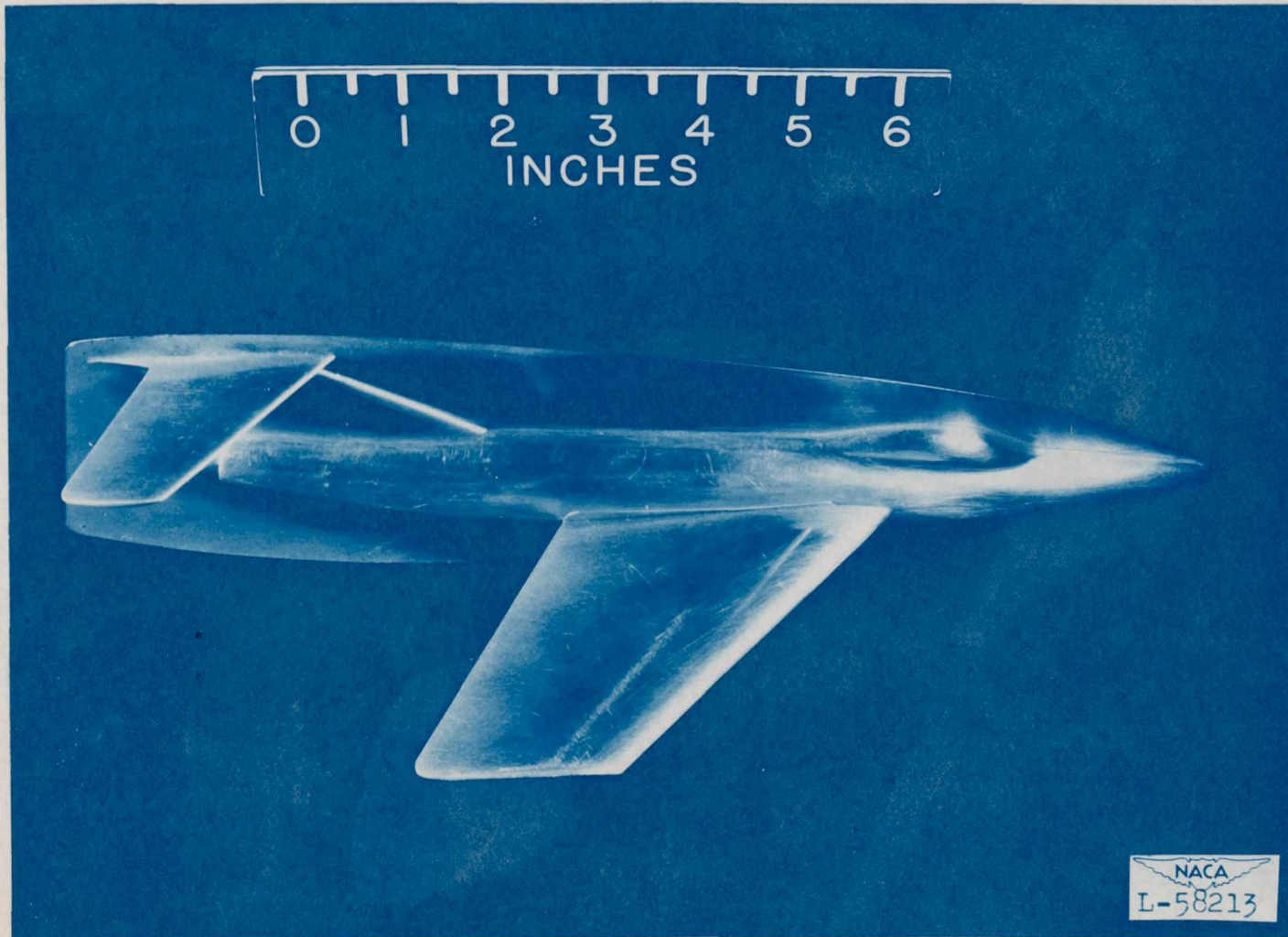
Figure 1.- Semispan model of the Grumman airplane design 83 equipped with a sweptback wing.
