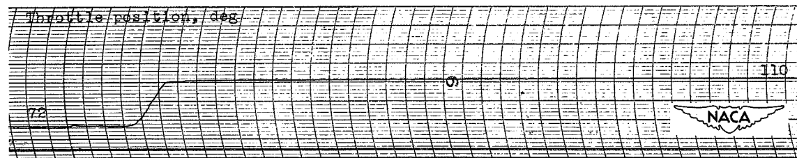
Figure 42. - Continued. Transient operation of automatically controlled engine with afterburner. Throttle position, 72° to 110°; altitude, 45,000 feet; nominal ram pressure ratio, 1.4; boost pump inlet pressure, 18 pounds per square inch.
