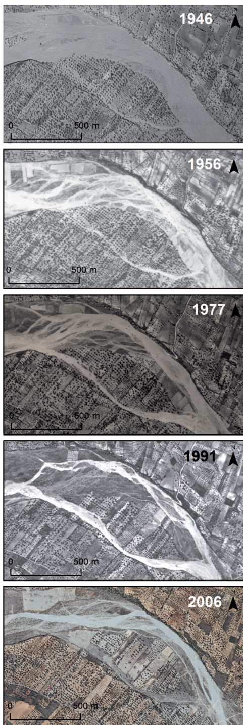
Figure 10. Evolution of a floodplain dissected island in the graben sector. A chute-channel dissected part of the floodplain during the flood of 1945. Subsequent events in the period 1956-1957 consolidated this channel form. Incision processes induced by gravel mining in the main gravel channel left the chute-channel lifted and, after the flood of 2000, it has been inactive. After 2006, part of the old channel has been planted with new olive groves.
