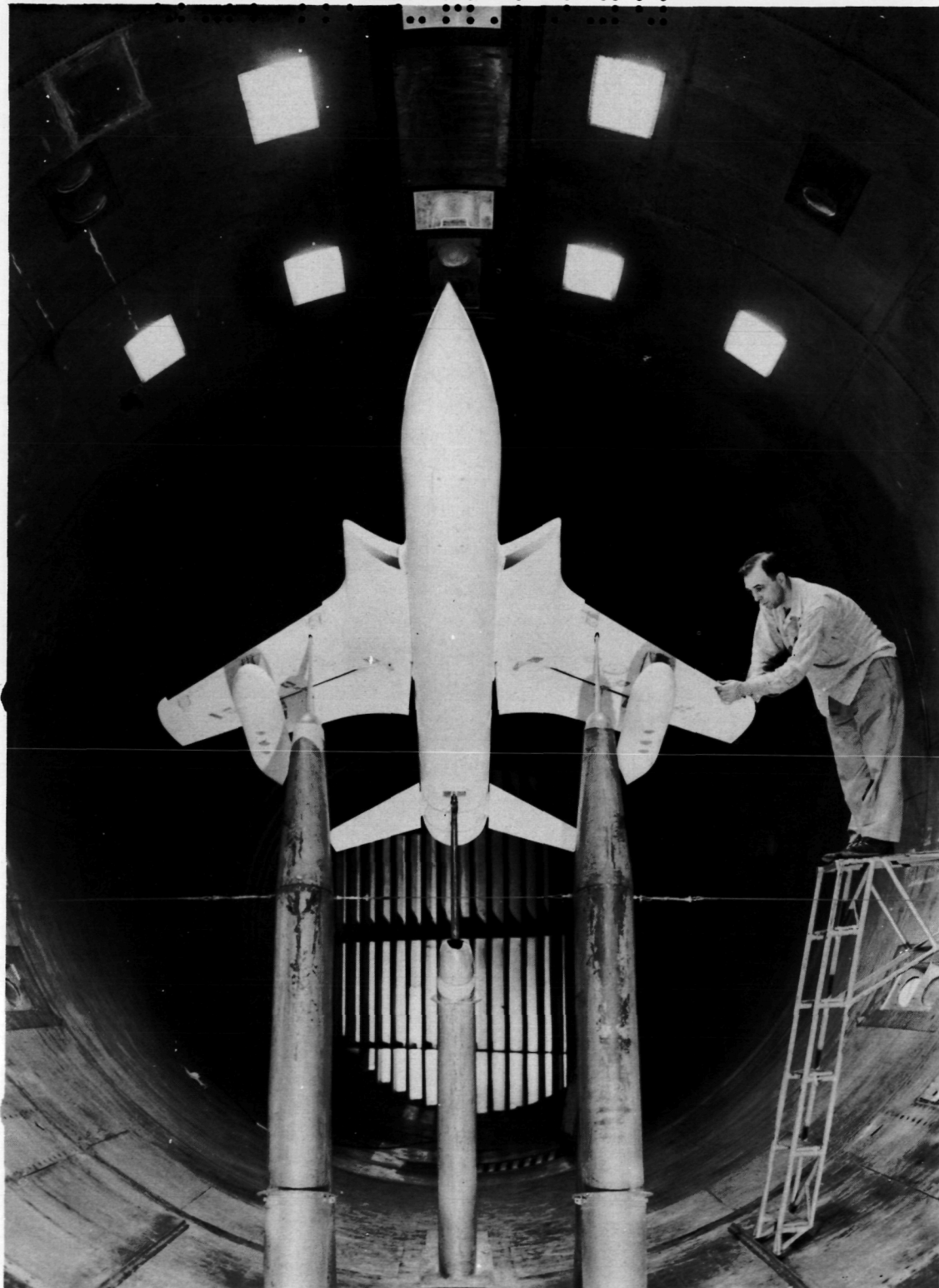
Figure 2.- The 1/4-scale model of the F-105 airplane mounted on the normal three-support system of the Langley 19-foot pressure tunnel.
