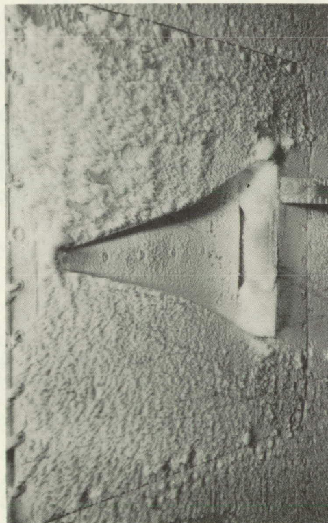
(b) Ice accretions on vent inlet after 60-minute icing time. Tunnel air velocity, 235 feet per second; tunnel-air total temperature, 21° F; liquid-water content, 1.1 grams per cubic meter.
