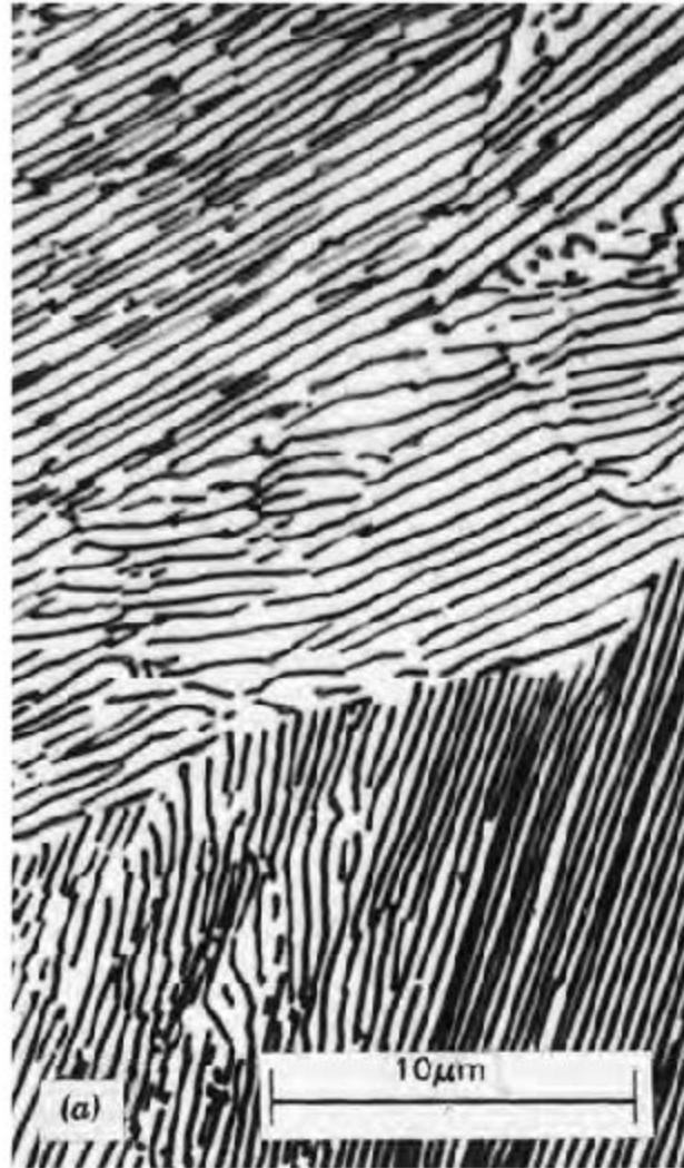
Figure 10.15 Photomicrographs of (a) coarse pearlite and (b) fine pearlite. 3000 \times . (From K. M. Ralls et al., An Introduction to Materials Science and Engineering , p. 361. Copyright © 1976 by John Wiley & Sons, New York. Reprinted by permission of John Wiley & Sons, Inc.)
