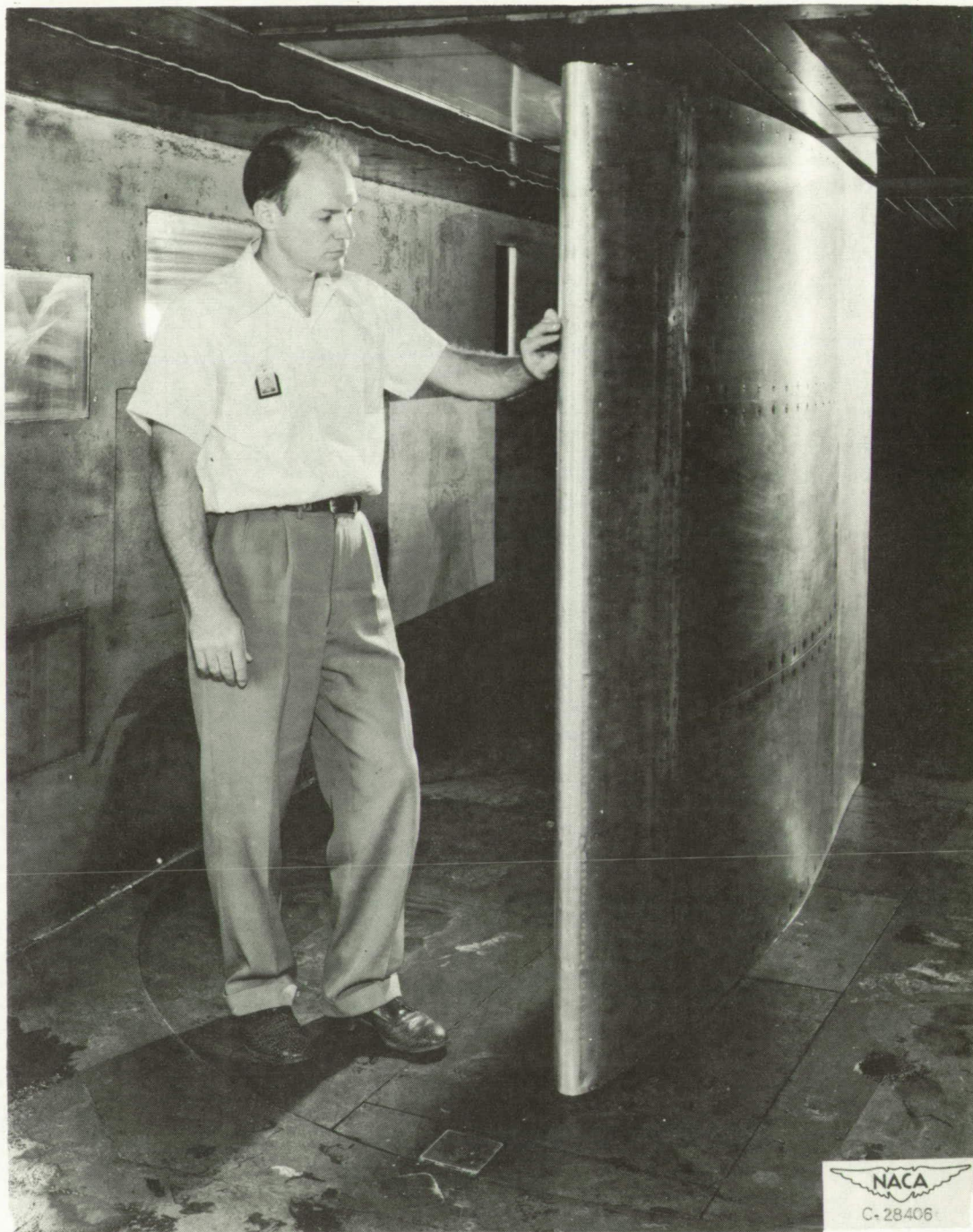
Figure 1. - Installation of airfoil model in 6- by 9-foot test section of icing research tunnel.
