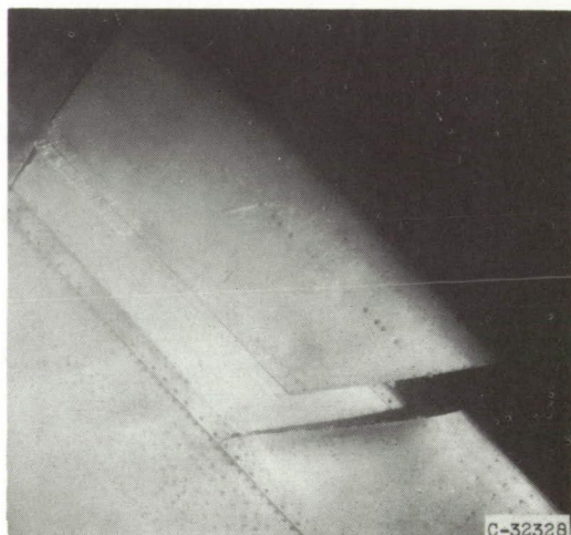
Upper surface. Icing time, 12 minutes; section drag coefficient, 0.0441; after ice removal.
