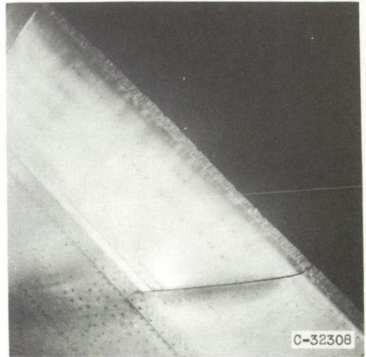
Upper surface. Icing time, 5\frac{1}{2} minutes; section drag coefficient, 0.0239.
