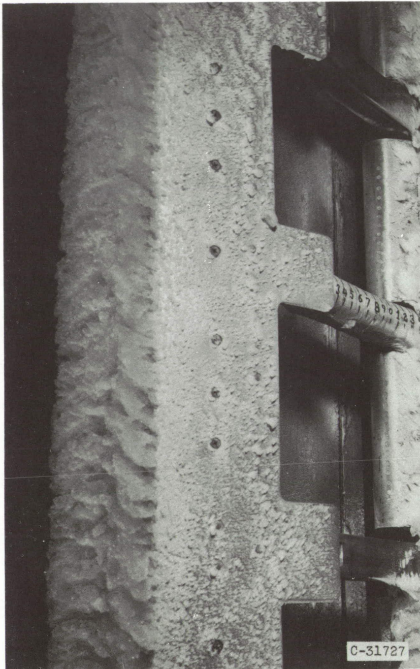
(d) Close-up of ice formations on slatted leading edge with 36^\circ sweep.
