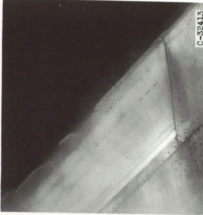
Upper surface. Icing time, 7\frac{3}{4} minutes; section drag coefficient, 0.0188; slatted airfoil.
