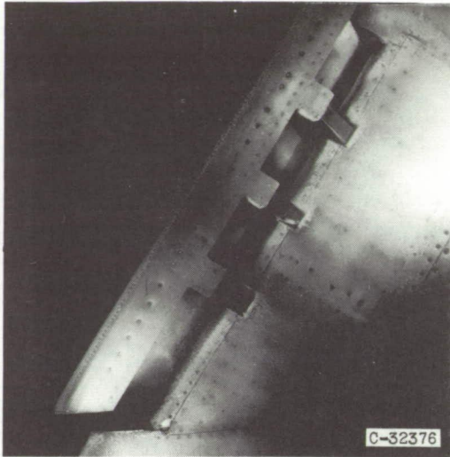
Lower surface. Icing time, 4 minutes; section drag coefficient, 0.0315.
