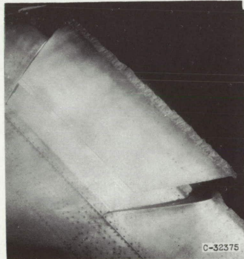
Upper surface. Icing time, 11 minutes; section drag coefficient, 0.0576.
