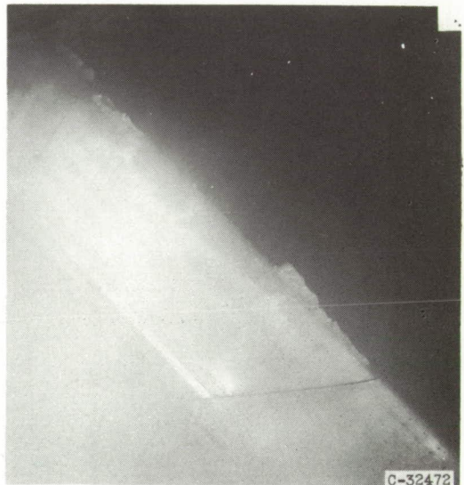
Upper surface. Icing time, 50\frac{1}{2} minutes; section drag coefficient, 0.0192.
