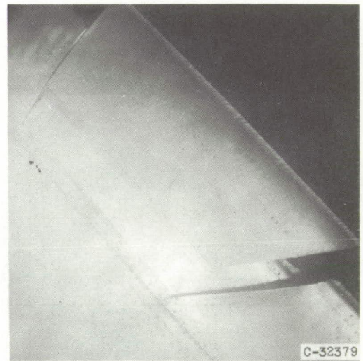
Upper surface. Icing time, 11\frac{1}{2} minutes; section drag coefficient, 0.0330.
