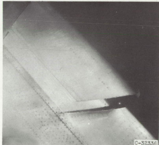
Upper surface. Icing time, 11\frac{1}{2} minutes; section drag coefficient, 0.0383; after ice removal.
