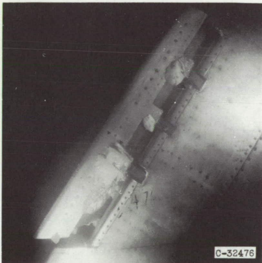
Lower surface. Icing time, 31 minutes; section drag coefficient, 0.0427.
