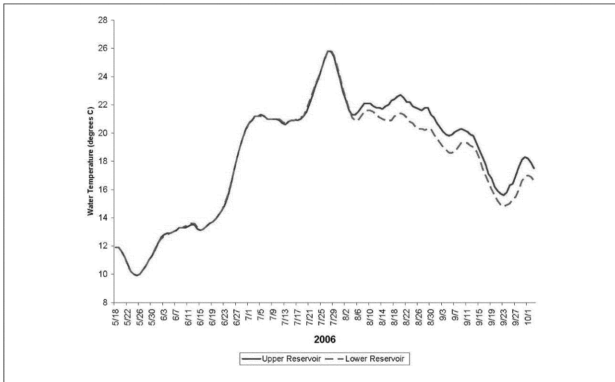
Figure 3. 7-DADMax temperatures in the lower end of the Enloe reservoir (RM 9.1) and at the upper end of the reservoir (RM 10.3) (Source: Okanogan PUD, 2008a).
