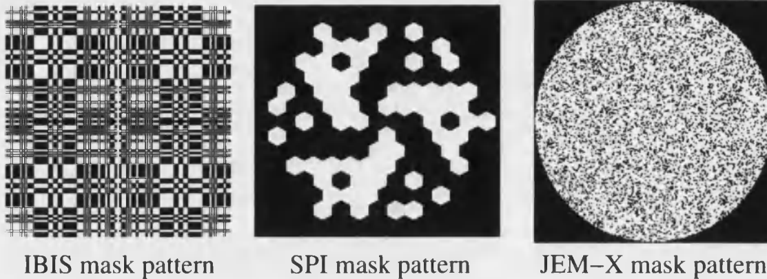
Figure 3.2: Mask patterns of the high energy instruments aboard INTEGRAL as used by the instruments software. Black zones denote those places with a zero value (i.e., transparent elements) while white zones correspond to elements with a value of 1 (opaque elements).
