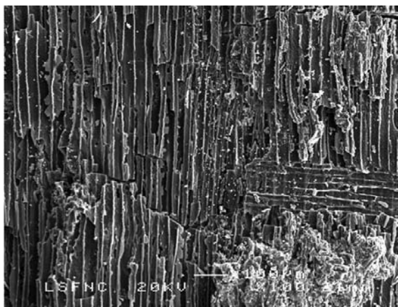
Figure 3. SEM image of the radial section of Pinus cf. pinaster/pinea from the North Profile. Conservation problems may be observed.
