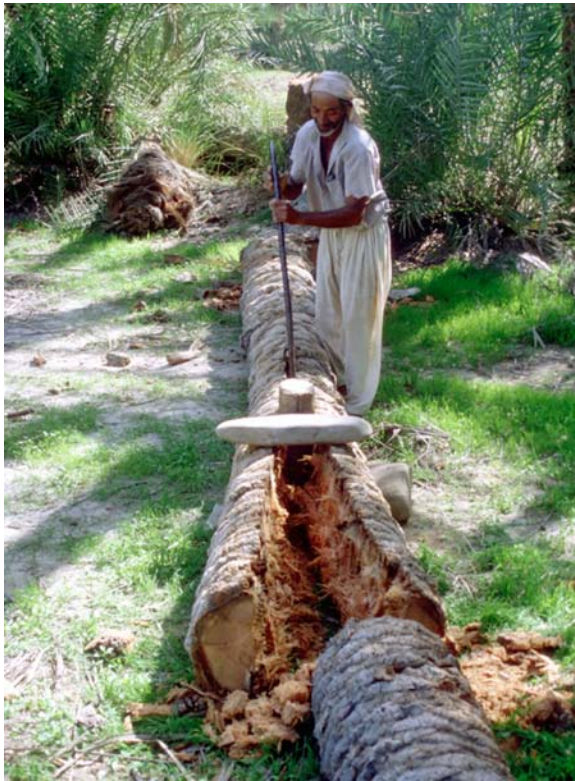
Figure 3. Beginning of the splitting of a date palm trunk for architectural purposes (Makran, Pakistan, © M. Tengberg).
