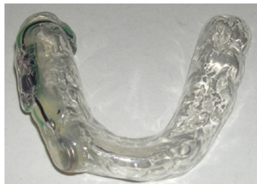
Fig. 1. The device is fabricated individually to lie on the lower dentition loosely. The electric circuit is embedded in the acrylic body. The stimulating electrodes are positioned in the area of the mandibular third molar, in proximity to the lingual nerve.
